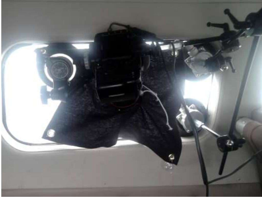
Figure 3. POV Camera (CANON EOS 5D Mark II equipped with Canon EF 24-105mm f/4L IS USM lens) showing the three-point suction cup tripod.
