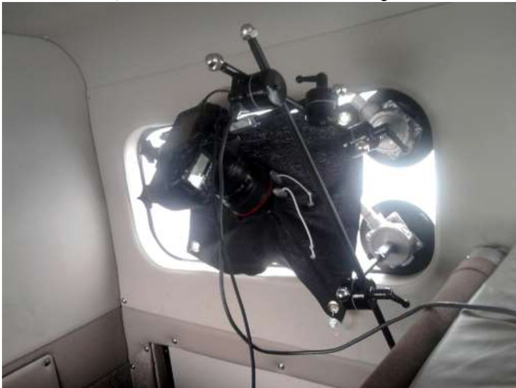
Figure 2. POV Camera (CANON EOS 5D Mark II equipped with Canon EF 24-105mm f/4L IS USM lens) configured to image the transect strip.
