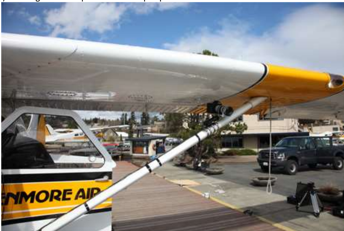
Figure 4. FF Camera. Wing strut mounted CANON EOS 5D Mark II equipped with Canon EF 70-200mm f/4L IS USM lens; lens is uncovered to show perspective.
