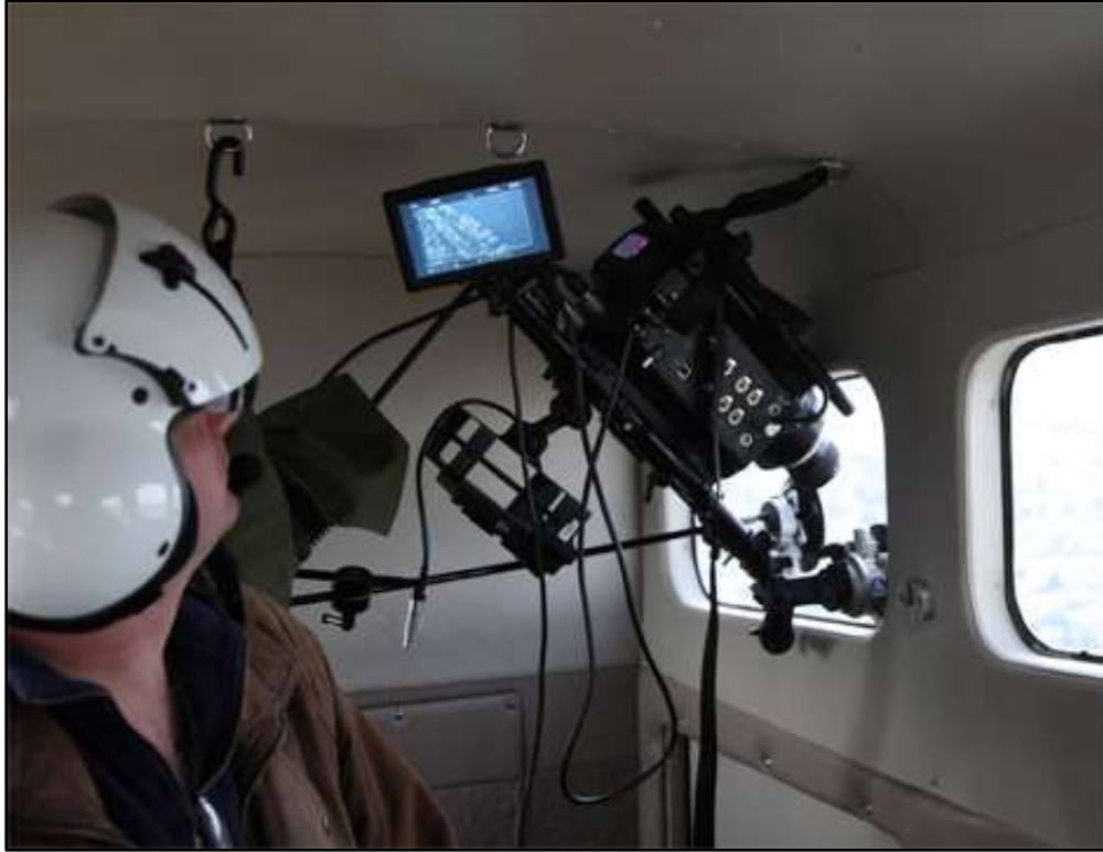
Figure 1. POV testing RedCam studio quality camera. With the suction cup mounting system, vibration was not an issue, even with a camera of this size and weight.
