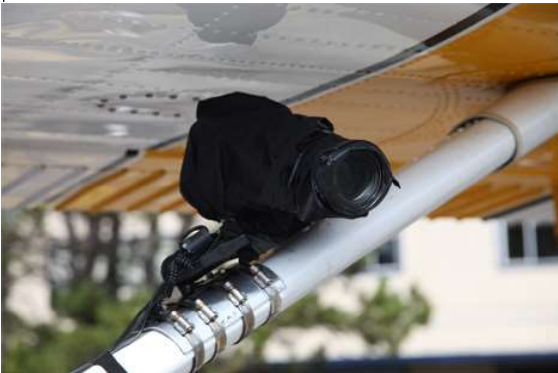
Figure 5. FF Camera. Wing strut mounted FF Camera (CANON EOS 5D Mark II equipped with Canon EF 70-200mm f/4L IS USM lens) showing protective cover over camera and lens.
