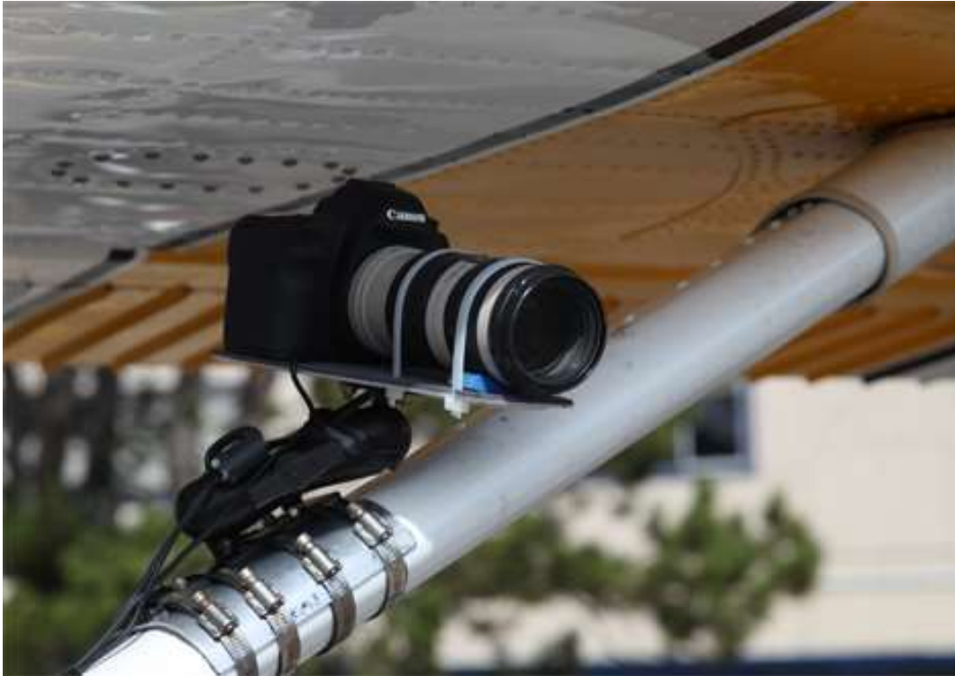
Figure 5. FF Camera. Wing strut mounted (Figure 2. POV Camera (CANON EOS 5D Mark II equipped with Canon EF 70-200mm f/4L IS USM lens) Camera and Lens is uncovered to show set up and attachment.
